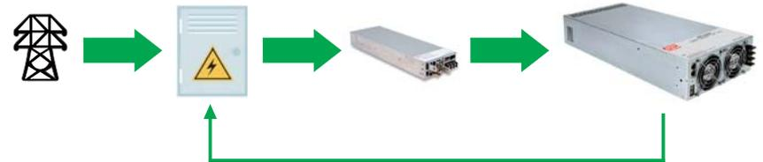
AC output voltage range of the ERG-5000 series is 200 - 240V/47 - 63Hz and its DC input voltage range covers DC: 10 - 420V, which is suitable for applications with different voltage requirement, such as equipment for battery discharge test and burn-in equipment for power supplies.
