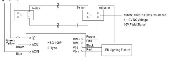
Using a switch and relay can turn ON/OFF the lighting fixture.
