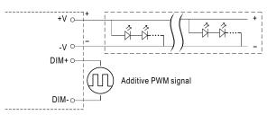
"DO NOT connect "DIM- to -V"
