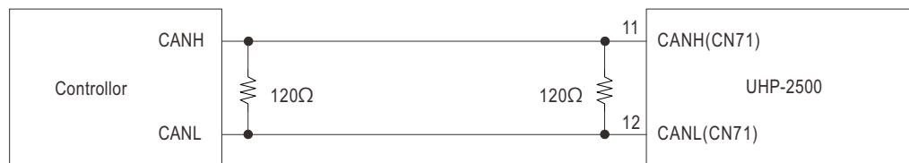
3. Communication function can be accessed immediately after UHP-2500 is connected to AC. First set it to communication mode.
