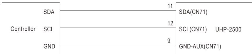
3. Communication function can be accessed immediately after UHP-2500 is connected to AC. First set it to communication mode.
